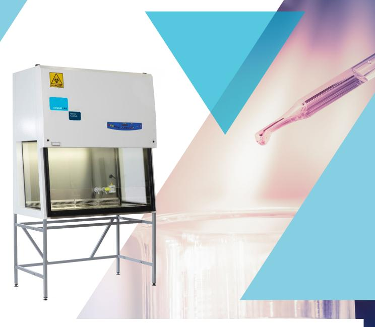
Envair SCS Evo Comfort + Class II Microbiological Safety Cabinets are designed and built to the performance requirements of the BS EN 12469: 2000 Standard, with 70% of the air re-circulated via the downflow H14 (EN1822) HEPA filter within the cabinet, whilst the remaining 30% is discharged through an exhaust H14 (EN1822) HEPA filter.
